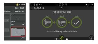
Follow the steps displayed on the screen in order to perform a calibration, then press on **Result.**
